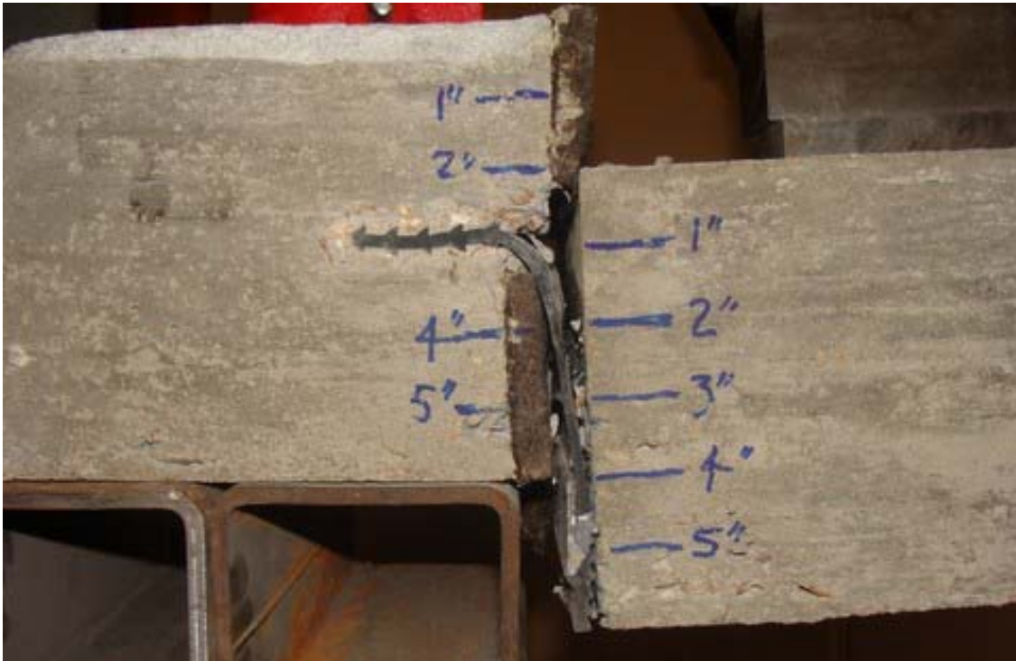
Figure 4.3 - Deflection approaching waterstop failure due to rupture in elongation
